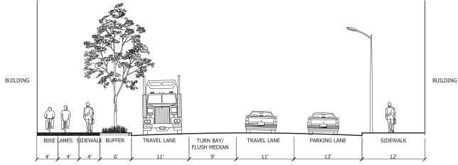
Fig. 9: Possible Configuration for Flushing Avenue
