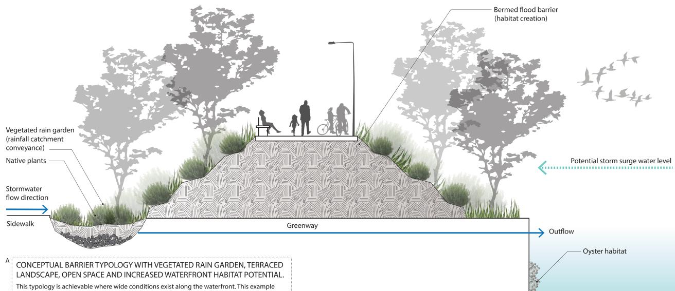
shows the potential for continuous vegetated rain gardens to manage upland stormwater runoff. Attractive vegetated terracing can increase habitat function and could capture and treat a large amount of rainfall.
