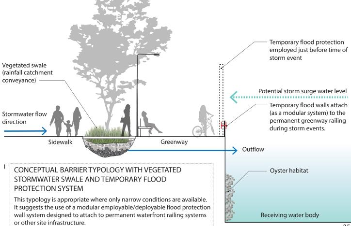
Temporary flood defense wall attached to permanent waterfront railing and pillar system.
