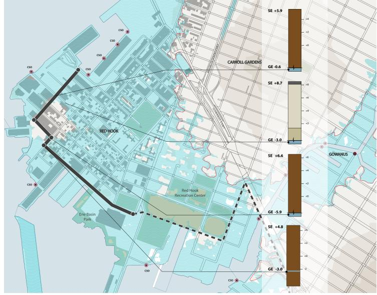
Figure 1: Red Hook (Segment 9) storm surge inundation area
